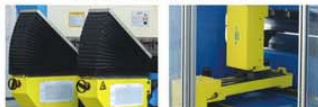
数控随动托料(选配) CNC following material holder (Option) 6轴后挡料(选配) 6-axis backgauge (Option)
